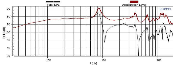
**Results:** The acceleration level is identical with the on-axis SPL response at lower frequencies where the cone vibrates as a rigid body. At higher frequencies we see the peaks in the acceleration level which occur at the natural frequencies of the mechanical modes.
