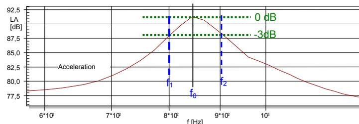
**Results:** The loss factor  $\eta$  is about 0.1 for the first natural mode occurring 850 Hz. To suppress the peak in the SPL response the loss factor has to be increased by factor 2 or more.
