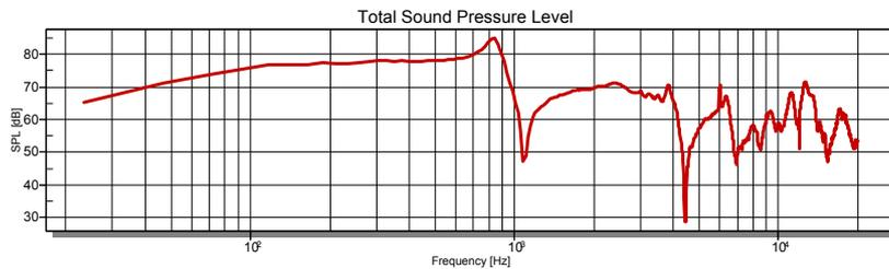
**Result:** The woofer under test has a flat response above the fundamental resonance (about 80 Hz) up to the 700 Hz. The significant peak at 800 Hz and the dip at 1100 Hz are not acceptable for the particular application.
