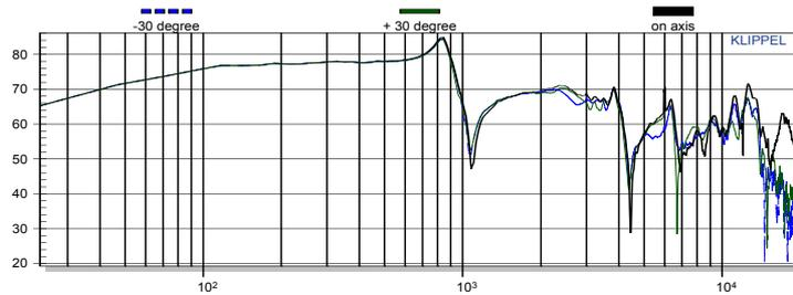
**Results:** The critical peak and dips appear also out of axis. Significant differences occur at higher frequencies.
