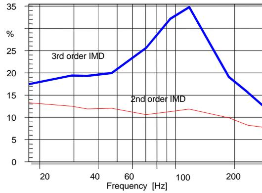
Fig. 9: 2<sup>nd</sup>- and 3<sup>rd</sup>-order intermodulation distortion according to IEC 60268-5 measured with a two-tone stimulus ( $15 < f_1 < 300$ ,  $f_2=1000$ Hz)
