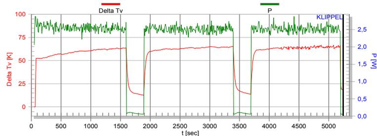
2. Activate the cursor by using the right mouse button and read the temperature of the coil  $\Delta T_{VSS} = \Delta T_v(t_{S\_ON})$  at the end of the ON-phase  $t = t_{S\_ON}$ . Ensure that the driver is in the thermal equilibrium by comparing the  $t_{SW\_ON}$  with the final temperature of previous ON-phases.
