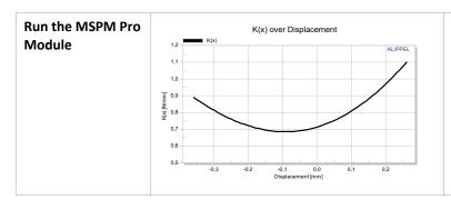
Data is extracted automatically from former measurements and the results are shown.
