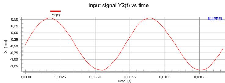
The waveform of the displacement reveals a dynamically generated DC part of -0.43 mm whereas the corresponding AC part is 0.7 mm rms.
