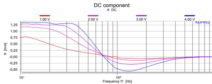
The speaker in the example produces both a positive and negative DC component depending on the frequency of the excitation tone. The crossing point at 70 Hz is close to the resonance frequency of the loudspeaker. These are typical characteristics for a motor with asymmetric  $Bl(x)$  characteristic. Shifting the rest position of the coil to positive displacement (out) would increase the  $Bl(x=0)$  value and improve the stability of the driver.
