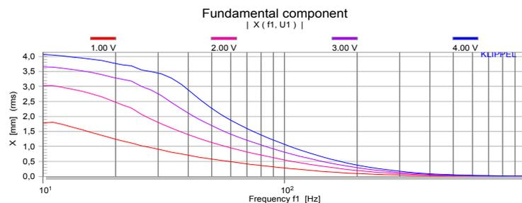
Due to the linear spacing of the input voltage the amplitude responses are equally spaced in the small signal domain. At low frequencies there is a amplitude compression at high signal amplitudes due to the nonlinear mechanisms.
