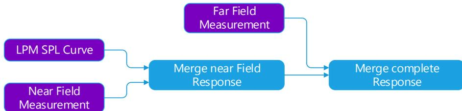
**How to do it:** Select the LPM Measurement: 3 LPM with accurate  $S_d$  and enter a very accurate  $S_d$  and the drivers nominal impedance in the property page *driver*.
