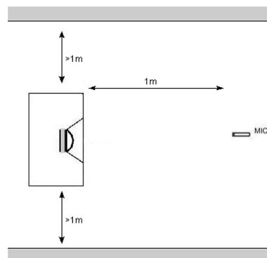
Usually the far field response of loudspeakers is measured at a distance between 1m distance.
