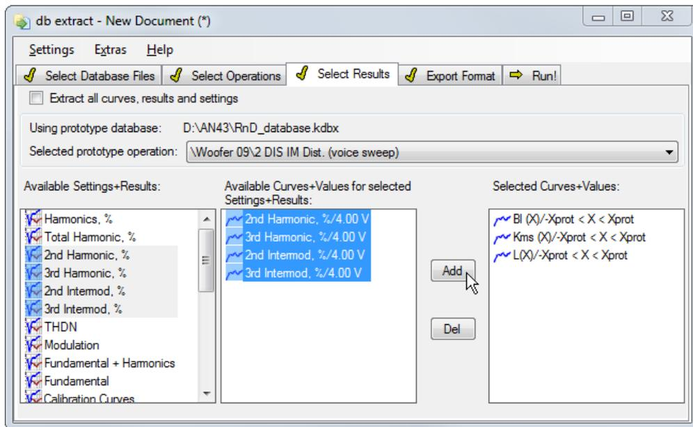
To select the Multitone Distortion Curve, choose any LPM Operation from the dropdown box and add the curve.
