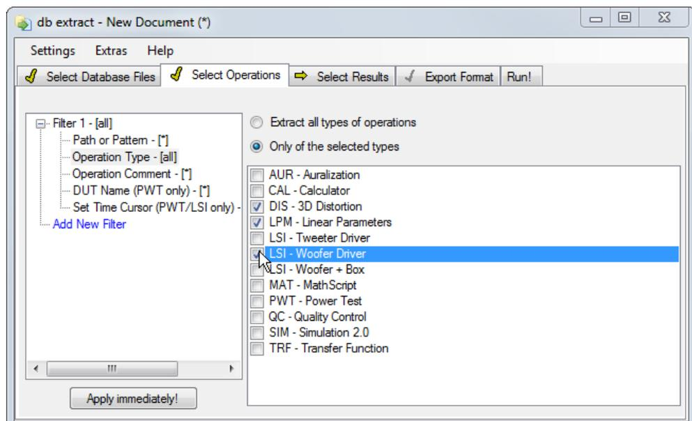
Using this filter, it is possible to select the type(s) of measurement operations we want to export. As described above, we are only interested in DIS, LPM and LSI – Woofer measurements. Using this filter will avoid extracting data from other operation types by accident if undesired operations are included in the input data.
