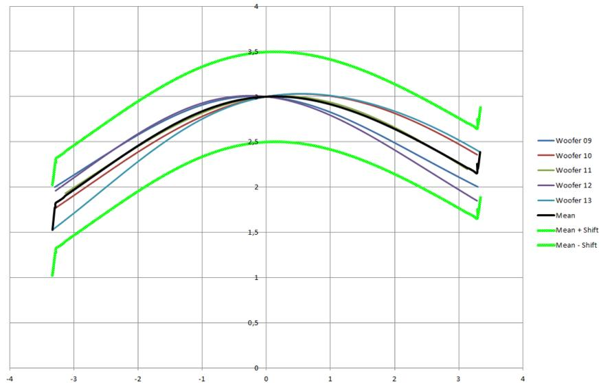
On the 'Curves for dB-Lab' spreadsheet, the mean and the shifted curves are represented in dB-Lab / MAT-Lab compatible format.
