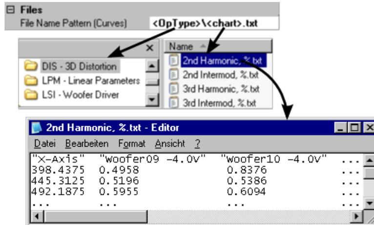
These examples are showing that the file name pattern allows defining how the curve data is stored in the file system structure. It is possible to create folders, subfolders and text files. One text file can contain one or multiple curves of the same or different types.
