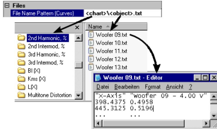
The "<OpType>\<chart>.txt" file name pattern generates a folder for each of the measurement modules (DIS, LPM and LSI). The folders contain one text file for each chart created by the corresponding module.
