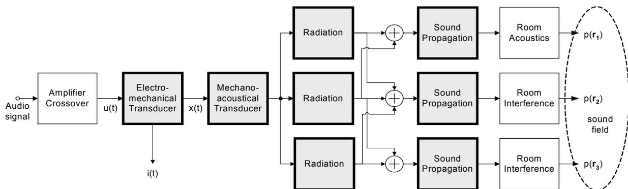
Fig. 1. Signal flow in a sound reproduction system
